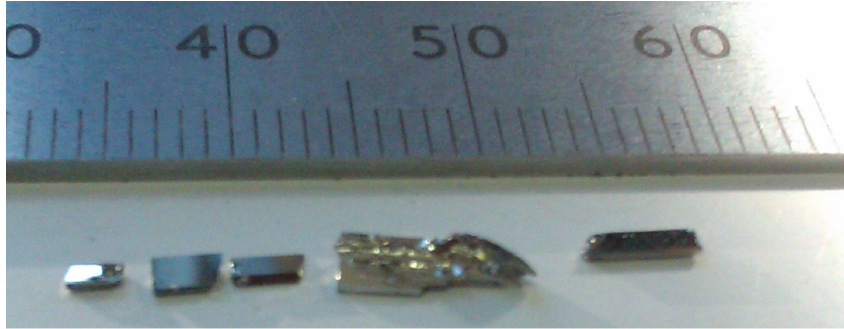
Figure 4.4: Photograph of several \text{CeCoGe}_3 crystals obtained using a flux method. A ruler is shown for scale where one division is equal to 1 mm.
