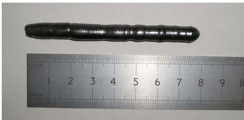
Figure 4.2: A \text{Co}_3\text{V}_2\text{O}_8 single crystal grown using the floating zone technique.
